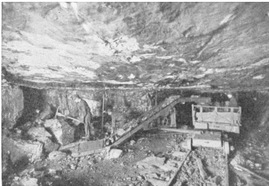
SCIENCE IN THE COAL MINE Portable Electric Loading Conveyor
